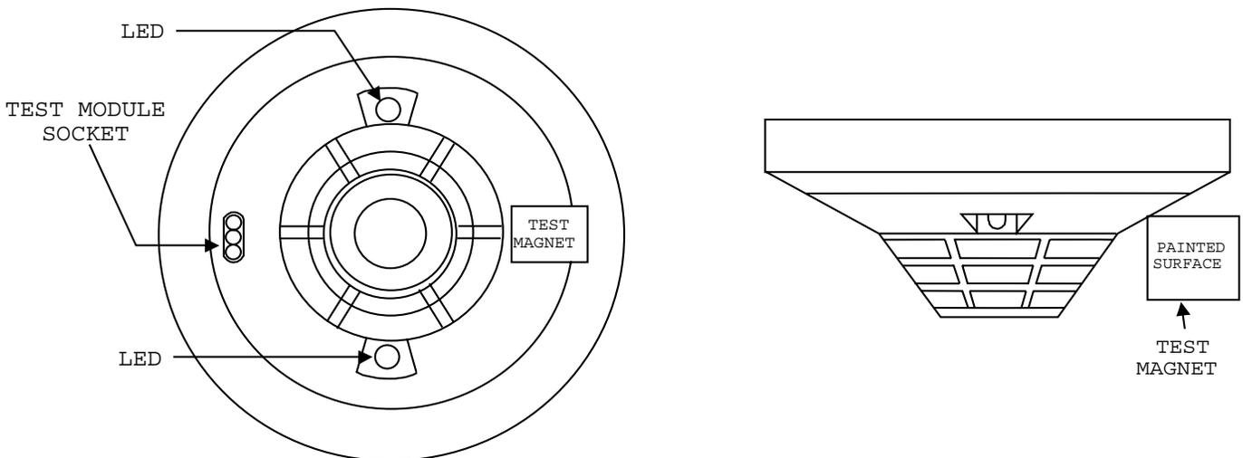
B. Test Module (System Sensor Model No. MOD400 or MOD400R)
